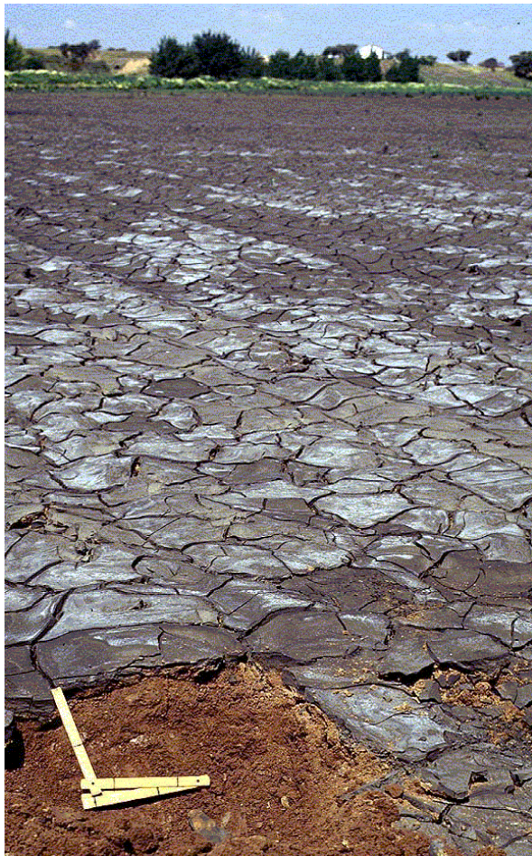
Figure 3.7. Sludge layer at Vado de Quemas, approx. 30 km downstream (from Aguilar et al. 2000). Note the bright efflorescent crusts on top of the sludge, which are the first oxidation indicators.
