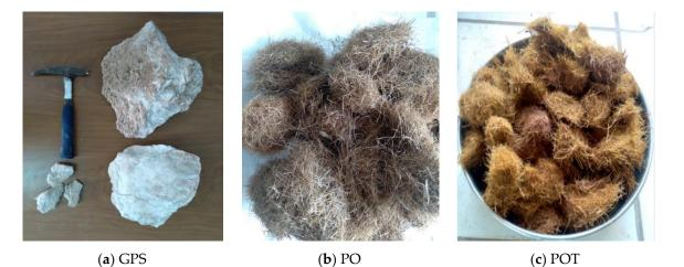
**Figure 1.** (a) The slices of gypsum (GPS), (b) Posidonia oceanic fibers (PO), and (c) the treated Posidonia oceanica fibers (POT).
