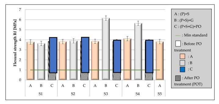
Figure 9. Variation in flexural strength of composites in the different mixing plans.
