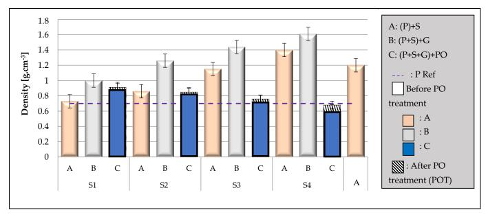
Figure 10. Variation in density of composites in the different mixing plans.
