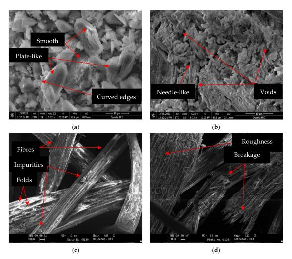
**Figure 6.** SEM images of (a) gypsum, (b) plaster, (c) Posidonia oceanic fibers (PO), and (d) POT with magnification of (a)  $7031 \times$ , (b)  $8324 \times$ , (c)  $488 \times$ , and (d)  $422 \times$ .
