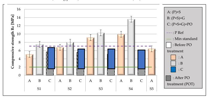
Figure 8. Variation in compressive strength of composites in the different mixing plans.
