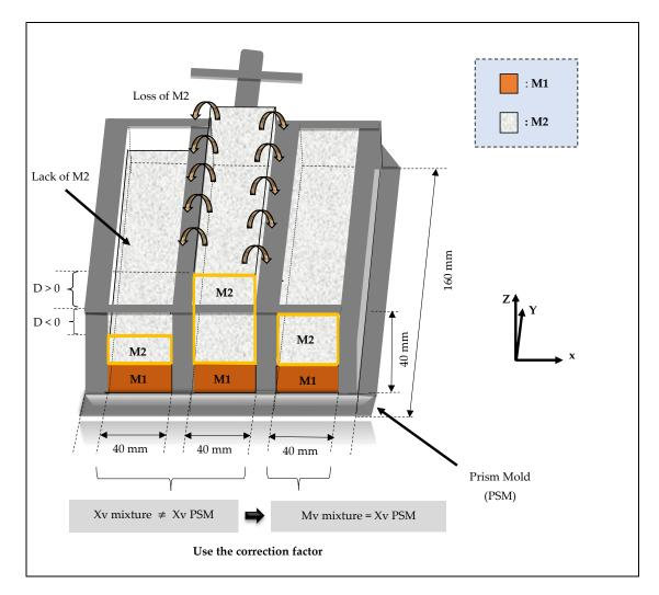
Figure 2. Pouring into molds before and after using the volume percentage correction factor.
