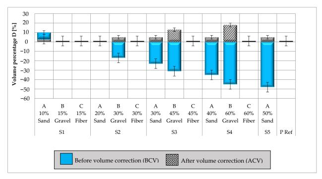
**Figure 3.** Comparison between the difference in volume percentage of mixture and prism mold 'D' before and after using the volume percentage correction factor.
