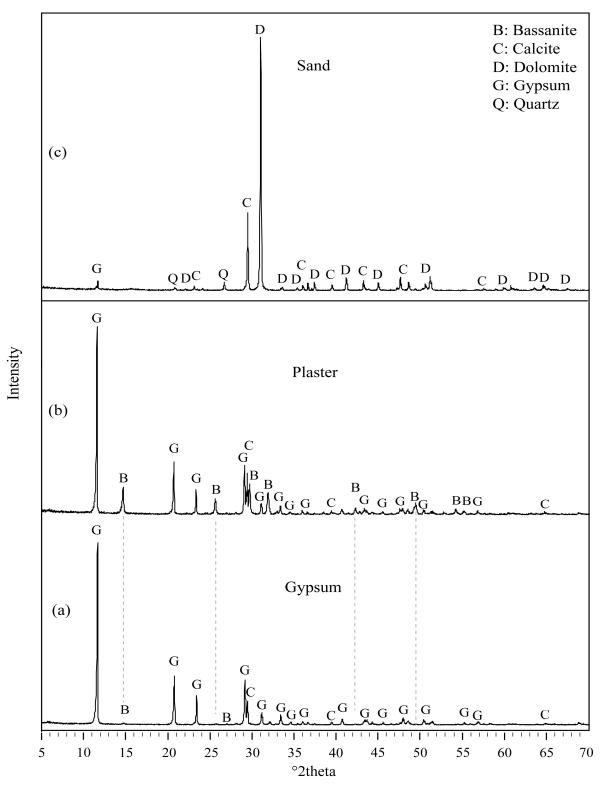
Figure 7. XRD pattern of (a) gypsum, (b) plaster, and (c) sand.
