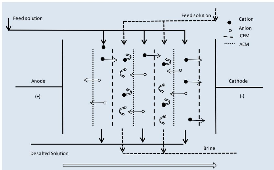
Figure 28: ED conceptual desalination process (sourced from Almadani, 2002)
