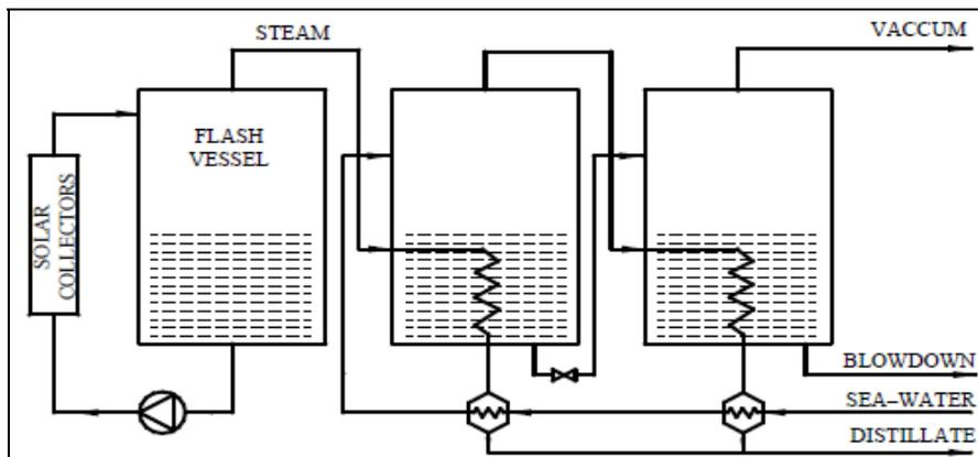
**Figure 18: MED solar collectors' process diagram (sourced from Kalogirou, 2005)**
