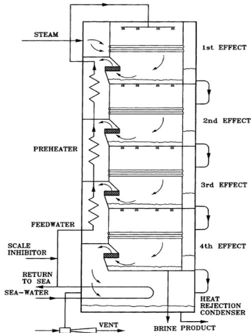
**Figure 19: MED process multi effect stack version diagram (sourced from Kalogirou, 2005)**
