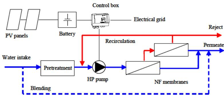
**Figure 27: Nano filtration flow diagram (sourced from Ghermadi et al, 2009)**
