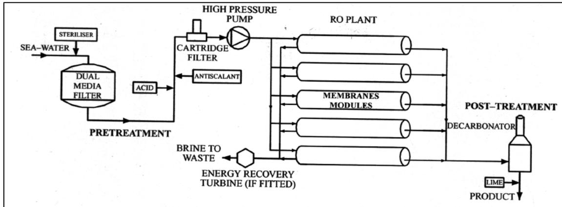
**Figure 25: RO process flow diagram (sourced from Kalogirou, 2005)**
