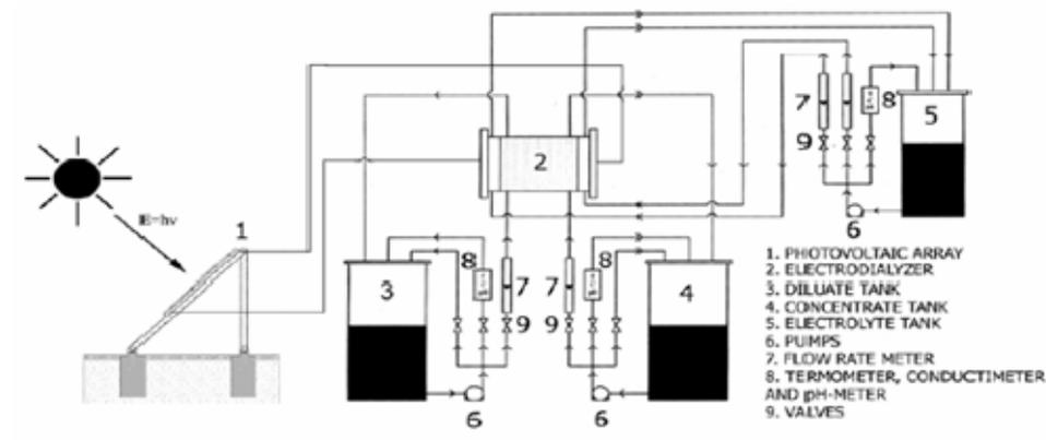
**Figure 29: ED process diagram (sourced from Ortiz al, 2005)**
