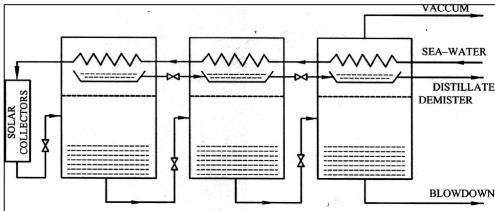
**Figure 17: Multistage Flash Flow diagram (sourced from Kalogirou, 2005)**
