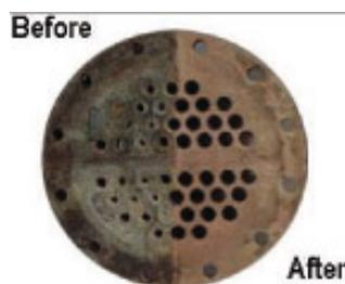
Figure 21: Tubes scaling blockages (sourced from Lenntech)
