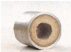
**Figure 30: Pipe scaling (sourced from [www.water.me.vccs.edu](http://www.water.me.vccs.edu))**
