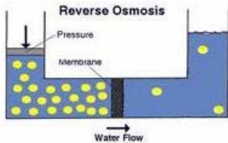
**Figure 26: RO process semi-permeable membrane ideal activity (sourced from membrane shop)**
