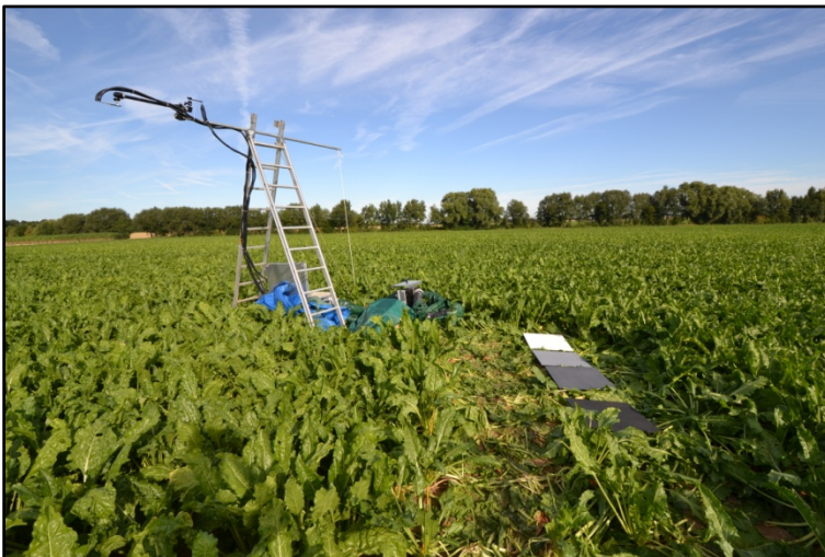
Figure 8.11 Field measurement setup at CKA2: field spectrometer and grey-level reference panels (Photo: M. Perez)
