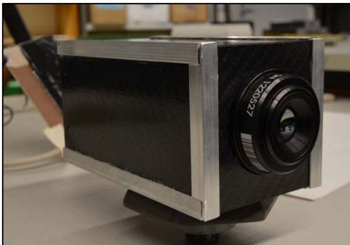
Figure 4.11 The thermal camera UCM (photo: G. Rock 2011)
