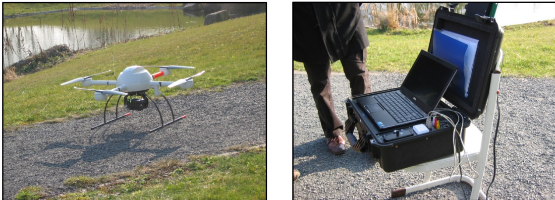
Figure 4.1 The md4-1000 with base station (photos: J. Besold 2011)
