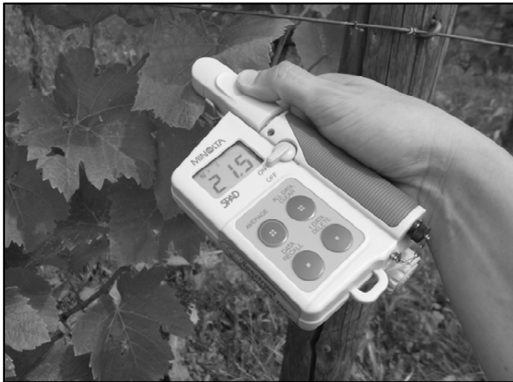
Figure 4.14 The SPAD-502 chlorophyll meter
