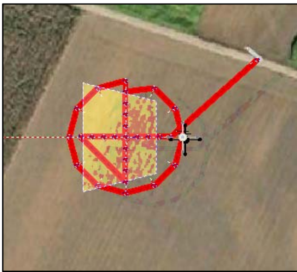
Figure 6.12: Goniometer-flight plan for maize field on the Ehranger Flur, Germany, presented on Google Earth data, image is oriented to the N (Google Earth: 28/04/2014)
