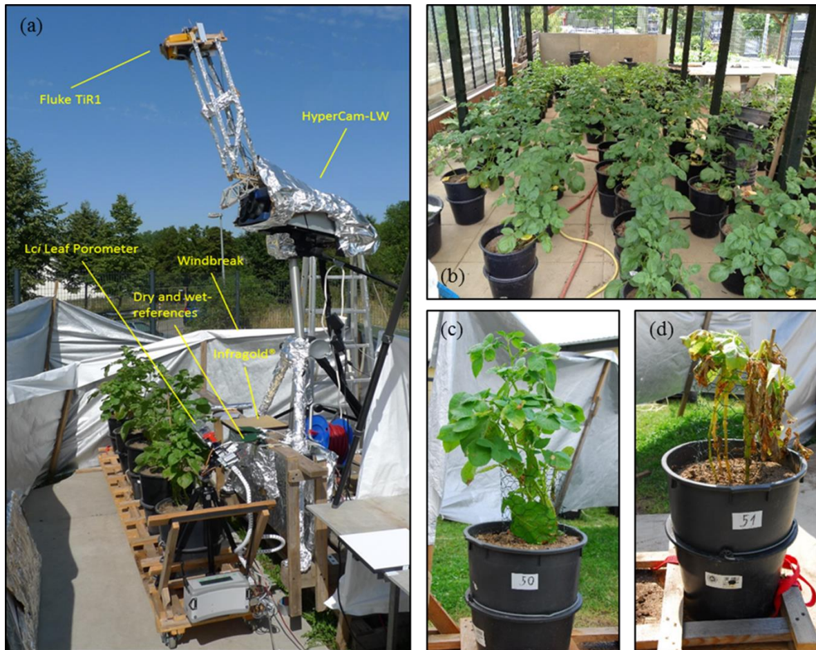
Fig. III-1: Experimental setup with Hyper-Cam LW on the tripod, Fluke TiR1, Lci leaf porometer, Infragold as well as dry and wet references targets (a), plant breeding and storage of the 60 potato plants under a roof construction (b), plants of the control (c) and treatment (d) group at day 9 after stress initiation.
