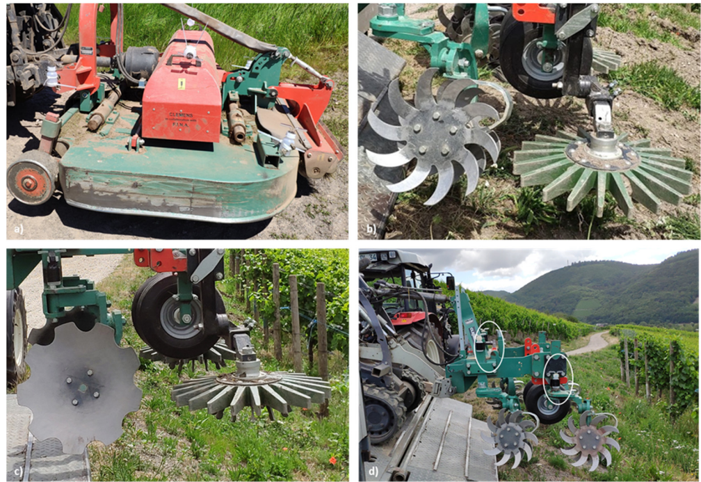
Figure 4. (a) Mulcher, (b) rotary-star tiller–finger hoe, (c) disc plough–finger hoe and (d) rotary-star tillers with equipped with MWAC samplers (marked).
