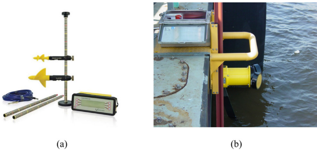
FIGURE 9.11 A current meter (Valeport Inc., UK, A) and an acoustic Doppler profiler (SonTek Inc., USA, B).
