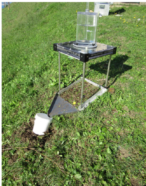
FIGURE 9.14 A rainfall simulator (Eijkelkamp, Nederland).
