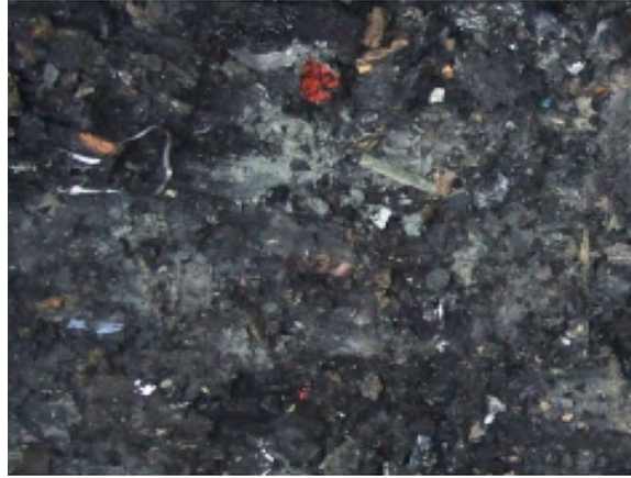
Figure A.1: The waste sample 1 (not sieved) from Muertendall was deposited before 1990. It has been covered with soil clay layer, thickness of 0.8 m. The sample has been taken out at the depth of 2.5 m. It was black and no smell of methane. The stabilized material has been noticed and documented.
