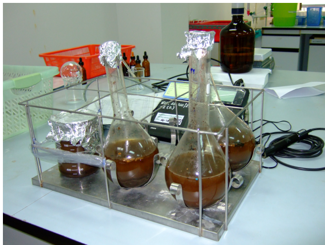
Figure 5.28: The extracted eluate in volumetric flasks by the standard procedure (1:10 solid/liquid ration and 24 hours shaking)
