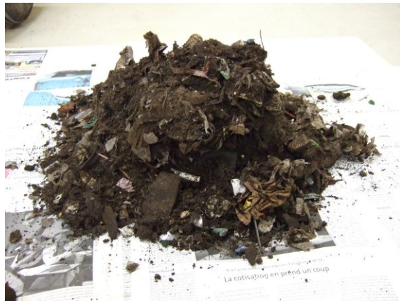
Figure A.8: The MBT waste, 35 weeks (not sieved) was dry, stabilized and less smell of methane. Its color was black.
