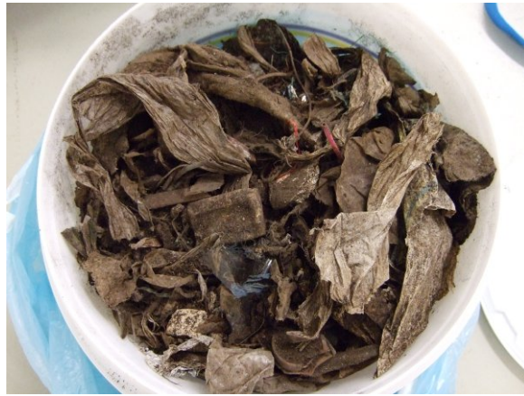
Figure A.5: The MBT waste, 20 weeks (not sieved) from Eiterköpfe. The waste was very dry, less smell, its color was brown and black. Not found composition of paper or large particles of plastics. They contained mostly of compost, seeds and corks.
