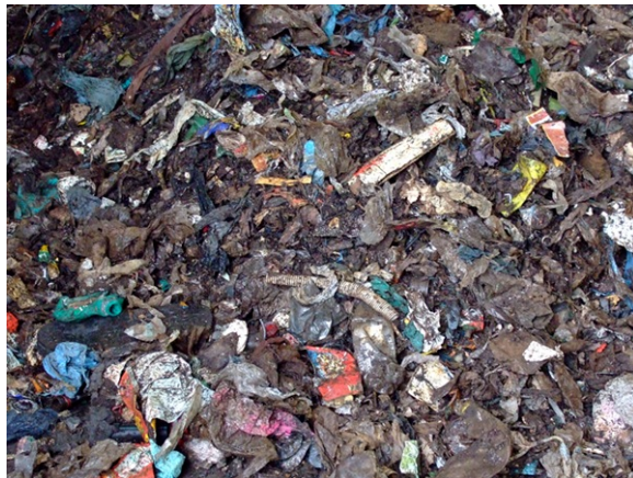
Figure A.4: The final MBT waste, 6 weeks (not sieved) from Fridhaff. The waste was moist, less smell of methane. They contained various kinds of waste component.
