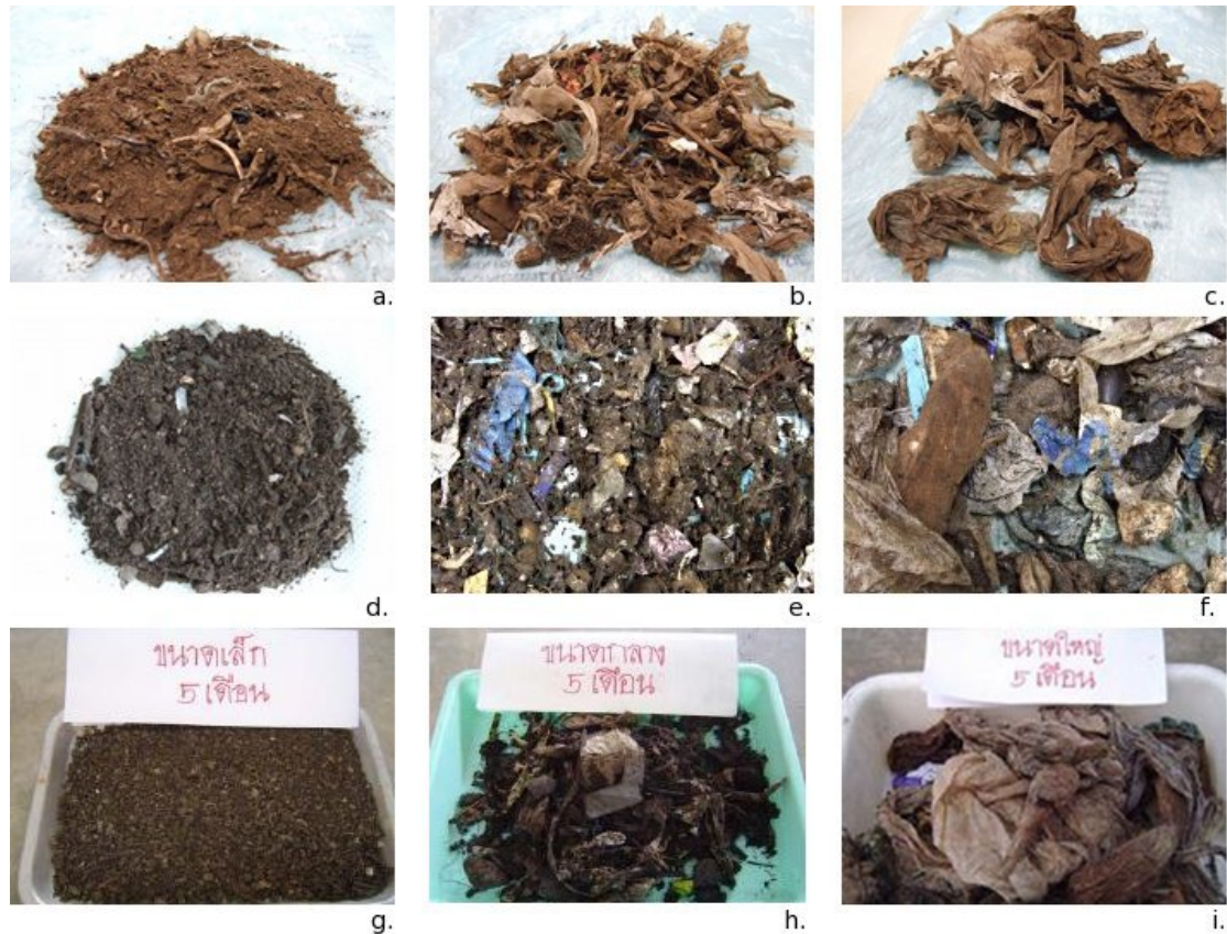
Figure 5.6: Images of three size fractions of MBT material analysis: a) small size < 10 mm of sample from Singhofen, Germany; b) medium size of 10 - 40 mm of sample from Singhofen Germany; c) large size of > 40 mm of sample from Singhofen Germany; d) small size < 10 mm of sample from Fridhaff Luxembourg; e) medium size of 10 - 40 mm of sample from Fridhaff Luxembourg; f) large size of > 40 of sample from Fridhaff Luxembourg; g) small size < 10 mm of sample from Phitsanulok Thailand; h) medium size of 10 - 40 mm of sample from Phitsanulok Thailand; i) large size of > 40 mm of sample from Phitsanulok Thailand
