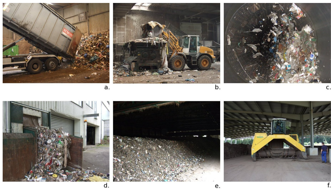
Figure 4.8: Mechanical and biological treatment of Linkenbach MBT plant in Germany: a) waste is delivered to the delivery hall; b) a small excavator put waste in the cutting machine/shredder; c) crushed material is screened inside screening drum with trommel sieve ca. 80 mm; d) high calorific potential material is separated and sent to thermal treatment; e) intensive rotting process at closed installation; f) second rotting process at the open installation
