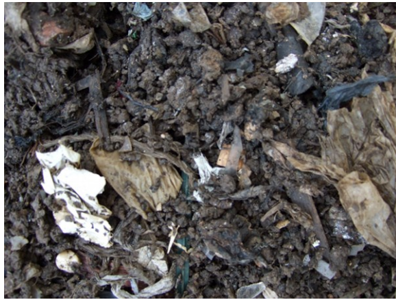
Figure A.3: The waste (1–2 years), (not sieved) the smell of methane was stronger. The waste sample contained living micro-organisms such as fungi and worms
