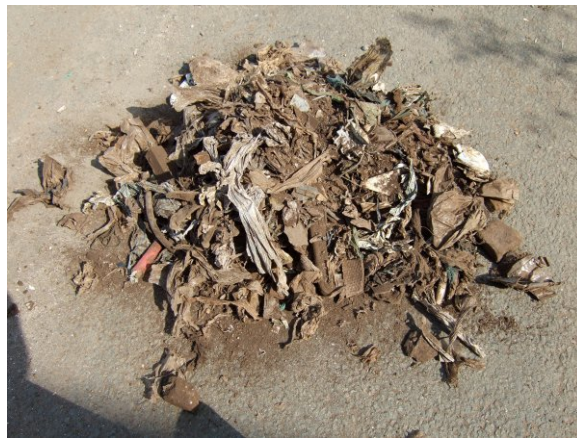
Figure A.9: The MBT waste, 15 weeks (not sieved) from Singhofen was very dry, less smell. Fine fraction could be seen by eyes.
