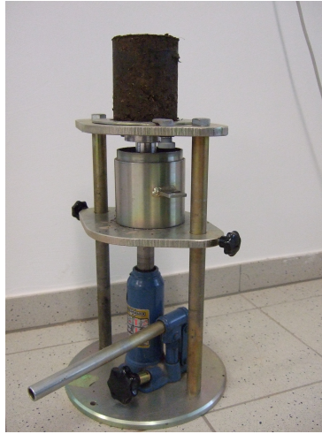
Figure A.11: MBT sample < 10 mm on extruder with manual hydraulic jack
