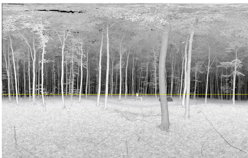
Fig. 2. Panoramic range image (2D-projection of single scan data). The yellow horizontal dash indicates the height above ground of the scanners' beam emission point. (For interpretation of the references to color in this figure legend, the reader is referred to the web version of this article.)
