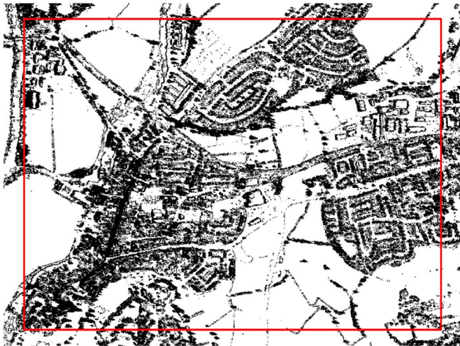
Fig. 10. Mask of regions unseen by TerraSAR-X due to shadow and layover, from [11].
