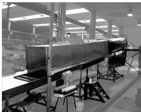
Fig. 2. Portable wind and rainfall simulator mounted on laboratory flume.
