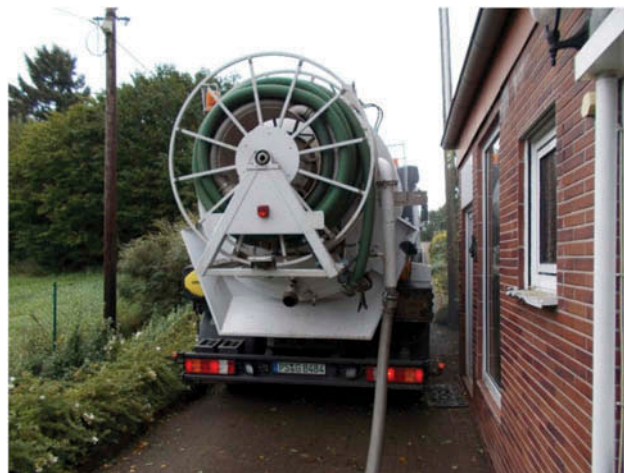
Figure 2. A wastewater pump truck services a septic tank (Photo City of Pirmasens).
